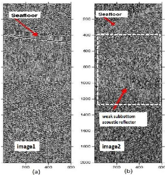
Figure 1. Subbottom profiler images at two offshore sites
