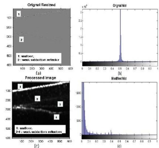
Figure 3. Image2 and its intensity histogram (a,b): before, (c,d) : after, segmentation process.
