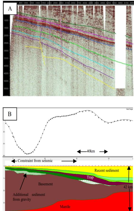
Fig.5 (A) Seismic section along profile 11' and (B) Gravity modeling of same profile.
