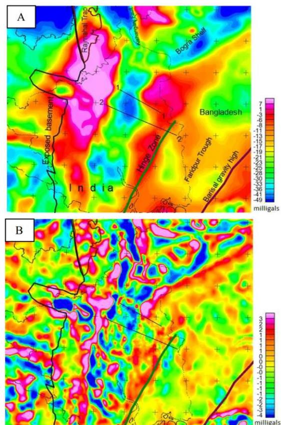
Fig. 3. (A) Bouguer gravity anomaly after merging with public domain Bangladesh gravity data. (B) Residual gravity data after a high pass filter of wavelength  $\leq 40$  Km.
