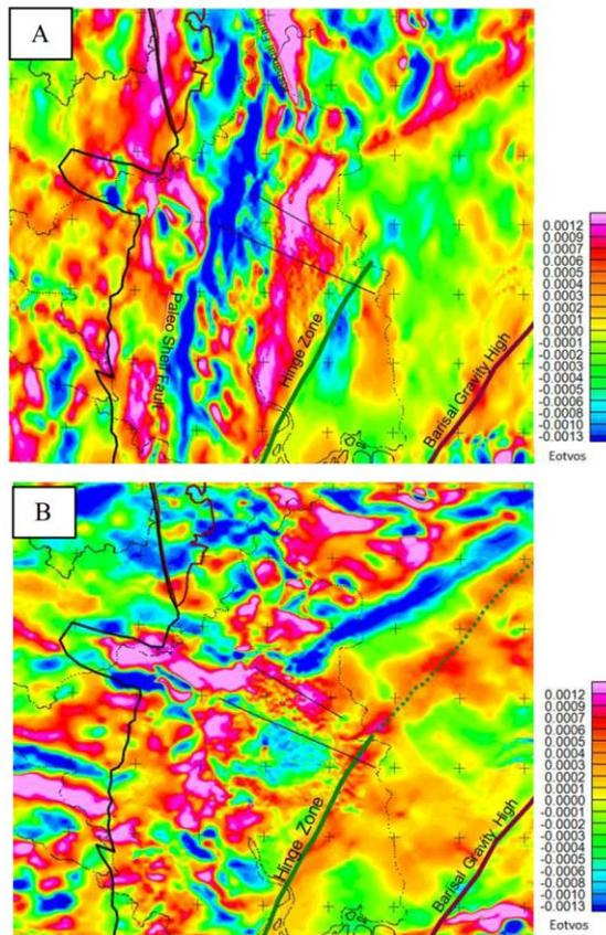
Fig. 4. Horizontal derivatives of Bouguer gravity anomaly (A) along East-West direction. (B) along North South direction.
