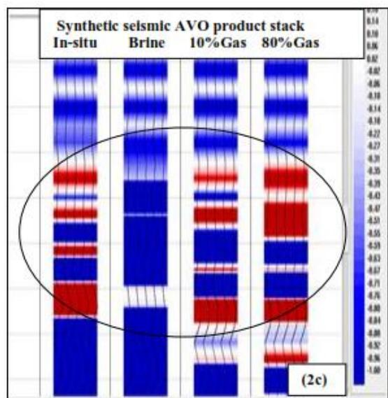
Fig. 2 (a) AVO Product stack passing through wells (b) Fluid Replacement Modeled logs for various scenarios (c) Synthetic-Sesimic AVO product stack (Intercept\*Gradient) using FRM logs
