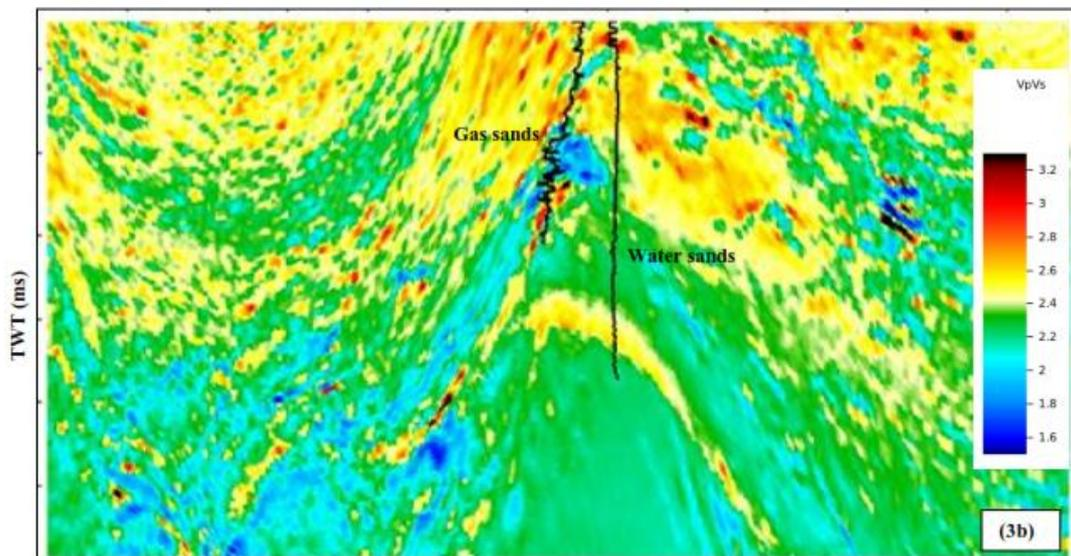
Fig. 3 (a) Comparison of inversion results with up scaled logs at well location (b) Inverted VpVs section passing through wells.
