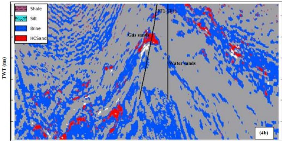
Fig. 4 (a) Probability density function of Poisson Impedance x VpVs from well logs (b) Section of most probable litho facies passing through wells
