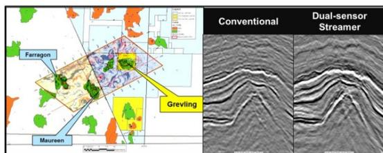
Figure 3: The left hand-side represents the location of the MultiClient survey over few North Sea fields including the Farragon and Grevling fields. The right hand-side panel shows the comparison between the conventional seismic and the dual-sensor seismic over the Upper Jurassic Grevling field. The dual-sensor streamer seismic exhibits a significant increase bandwidth.
