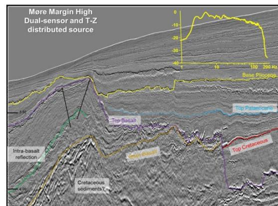
Figure 2: the figure represents a portion of a seismic line (Møre Marginal High, Norway) acquired with a dual-sensor streamer and depth-time distributed source-arrays. The amplitude (log scale) has been computed in the Pliocene interval and shows a frequency bandwidth from 2.5/3Hz up to 180 Hz. Previously not seen, intra-basalt reflections are now visible with this new dataset with also a good signal to noise ratio.
