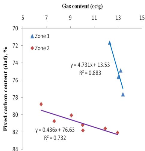
Figure 2: plot between gas content and fixed carbon content (daf)
