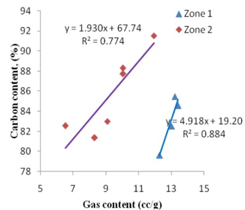
Figure 3: Relation between gas content and carbon content of coal
