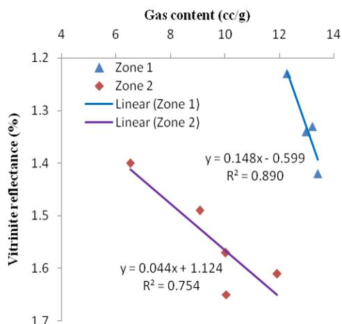
Figure 4: Plot between gas content and vitrinite reflectance
