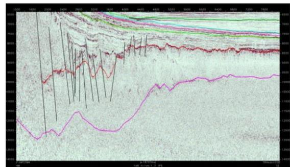
Fig.8 Seismic section passing through continental crust area indicated by series of horst-graben features
