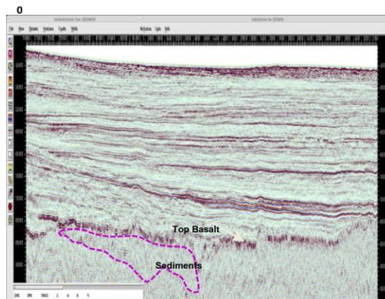
Fig.6 NW-SE seismic section from east coast of India up to 85°E ridge indicating rugged topography of basement
