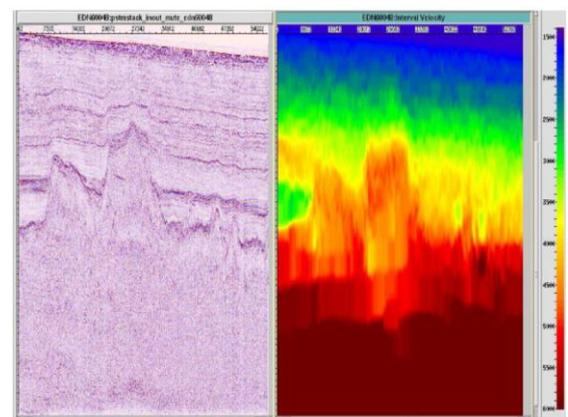
Fig.9 Comparison of Interval velocities along a seismic line passing through volcanic ridge
