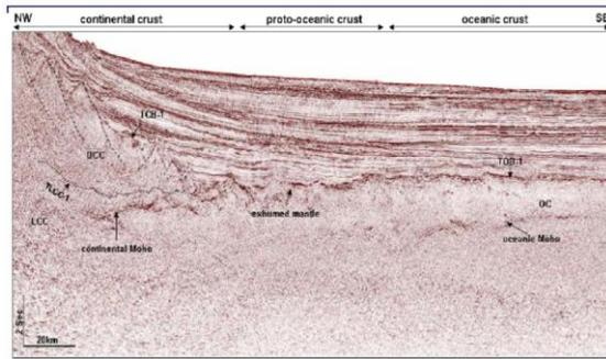
Fig.5 NW-SE seismic section from east coast of India towards east indicates the broad divisions of continental, transitional and oceanic crust areas.
