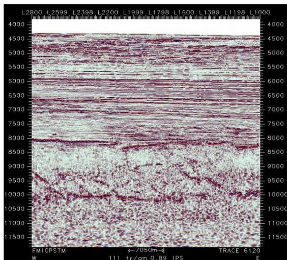
Fig.2. Q-Marine seismic data showing clear events corresponding to basement and mantle-crust boundary
