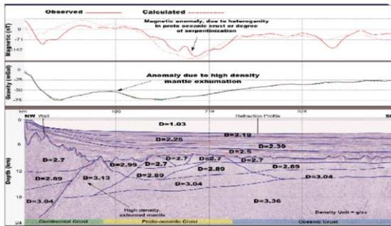
Fig.10 Gravity-Magnetic model along a NW-SE section showing a good fit between observed and calculated anomalies
