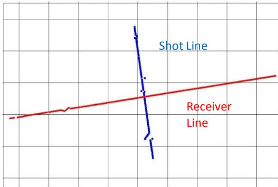
Figure 2: A cross-spread layout
