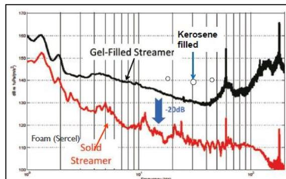
Figure 2. Streamer Noise Levels
