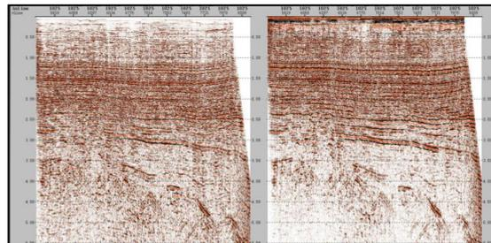
Figure 6: Stack response -without deghosting (left) and with deghosting (right)
