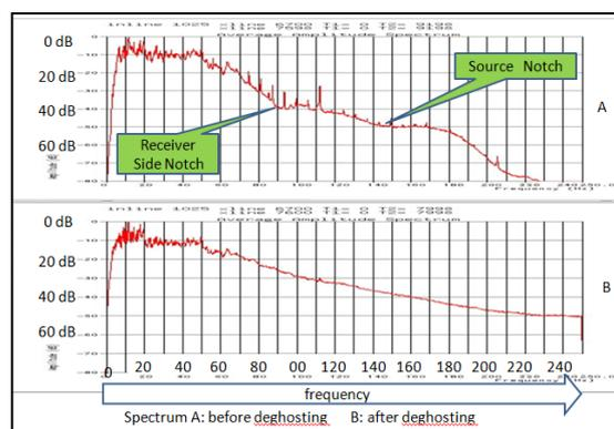
Figure 7: Spectrum before de-ghosting (top) and after de-ghosting (bottom)
