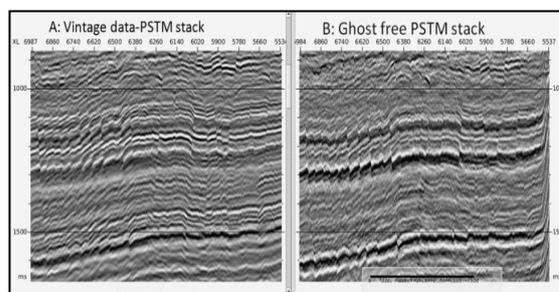
Figure 9: Comparison with the legacy data processed without de-ghosting (left) and newly acquired data processed in broadband sense (right)
