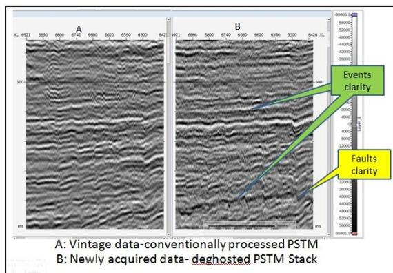
Figure 8: Comparison with the legacy data processed without de-ghosting (left) and newly acquired data processed in broadband sense (right)
