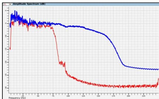
Figure 11: Comparison of spectrum on PSTM Stack section of legacy data processed without deghosting (red) and newly acquired data processed in broadbandwidth sense (blue)
