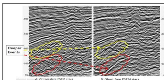
Figure 10: Comparison with the legacy data processed without de-ghosting (left) and newly acquired data processed in broadband sense (right)
