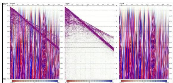
Figure 4: Raw Shot gather (left) and after low cut filter (1-2 Hz) (mid) and their difference plot (right)
