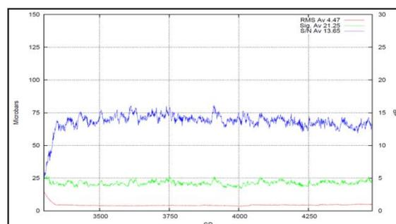
Figure 3: A graph of the shot averaged RMS noise, signal and signal-to-noise ratio.
