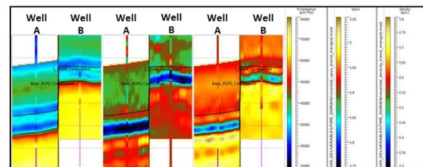
Figure 5: Inverted full bandwidth P-Impedance (left), Vp/Vs (middle) and density (right) around wells. Blue
