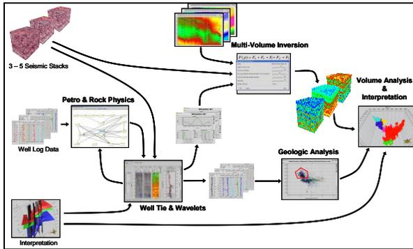
Figure 1: Standard workflow for simultaneous Inversion.
