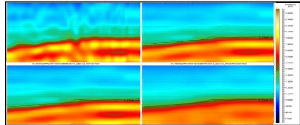
Figure 2: Section showing interval velocity from RMS velocity in a coarse grid (top left), interval velocity after application of median filter (top right), interpolation to seismic grid (bottom left) and high cut filter to (bottom right). Other two figures show intermediate steps.
