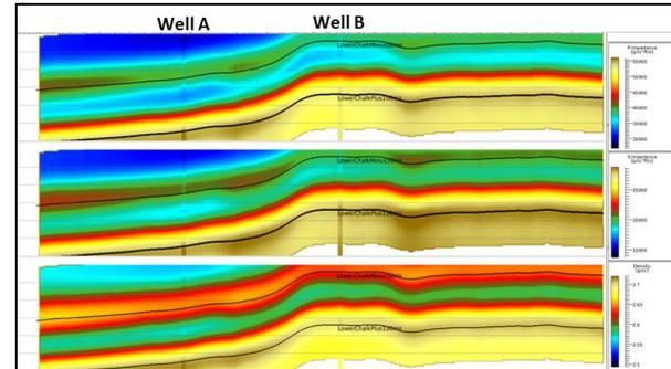
Figure 4: Section showing the Low Frequency models for P-impedance (top), Vp/Vs (middle) and density (bottom). Blue indicates lower value & golden-yellow indicates higher value.
