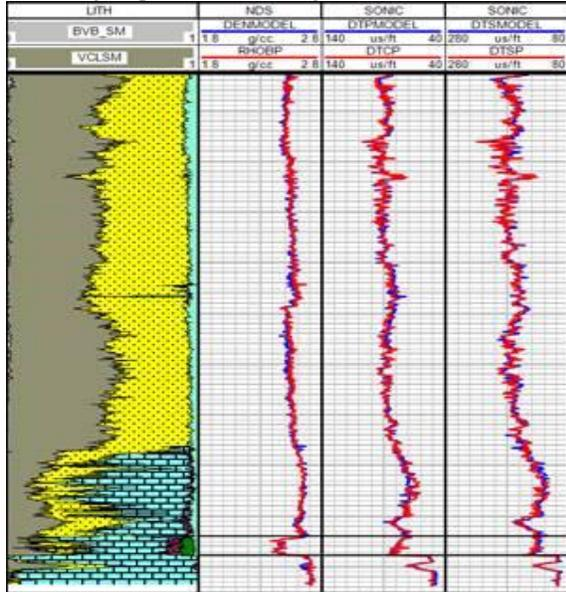
Figure 3: Comparison of measured logs (red) and modeled logs (blue) shown in last three tracks. The shear wave is shown in the last track.
