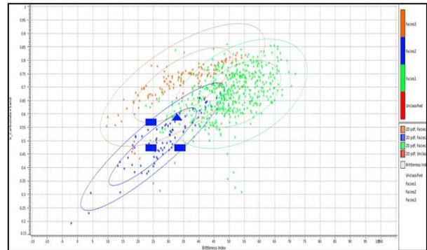
Figure 7: Cross plot of volume of carbonate and sands versus brittleness index coloured by facies. The pdfs corresponding to three different facies have been shown by different colors. Most brittle facies is represented by red.
