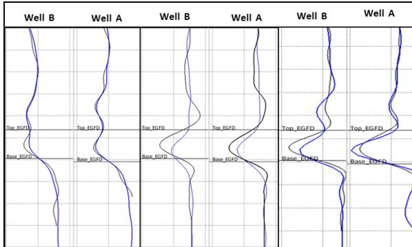
Figure 6: Inverted (Blue) and wireline (Black) P-Impedance, Vp/Vs & Density logs from left to right respectively.
