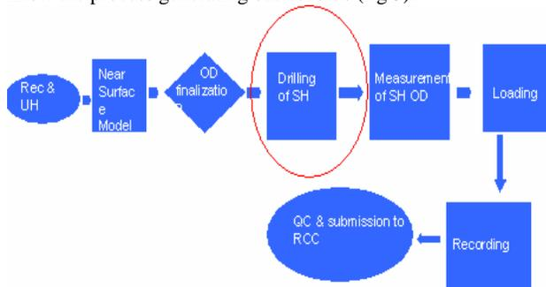
Fig 3: Macro Process Map of Seismic data recording
