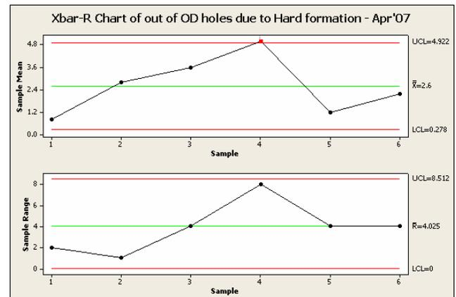
Fig 9: Xbar-R chart of out of OD holes for Hard Formation
