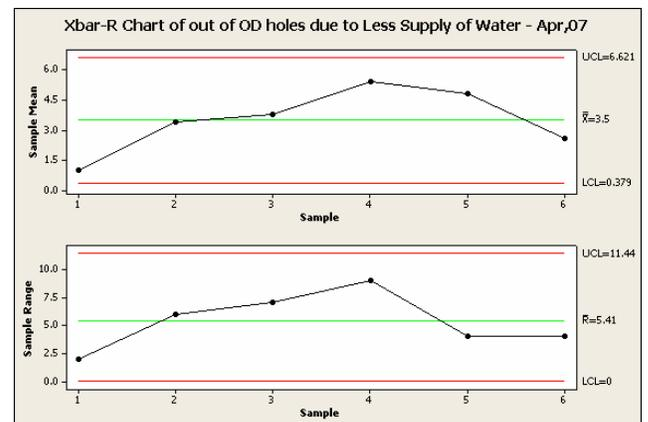
Fig 10: Xbar-R chart of out of OD holes for Less Supply of Water
