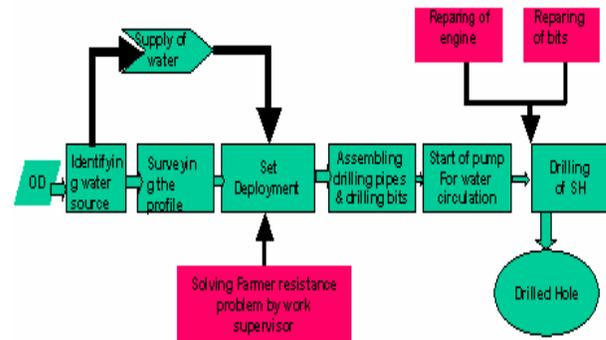
Fig 4: Detailed Process Map of Shot Hole Drilling
