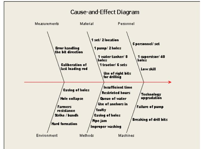
Fig 5: Cause and Effect (Fish Bone) diagram
