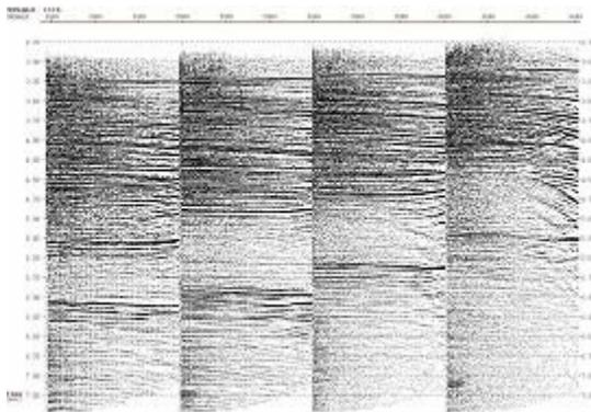
Figure -5 PSTM Gathers along Inline A showing Residual Moveout
