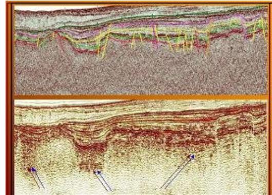
Fig-11: PSTM Stack of line no BB' showing Sub-basalt images
