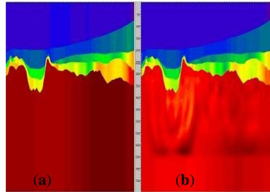
Fig-6 Interval Velocity- Initial (a) and after 1<sup>st</sup> Grid Tomography(b)
