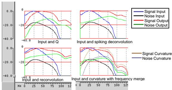
Figure 8: Signal & Noise spectrum comparison. Black & blue color respectively shows S&N spectrum of input.
