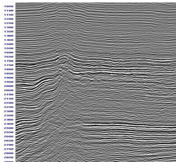
Figure 3: Stack after inverse Q filtering
