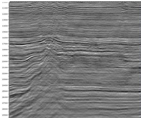
Figure 2: Stack after Spiking deconvolution
