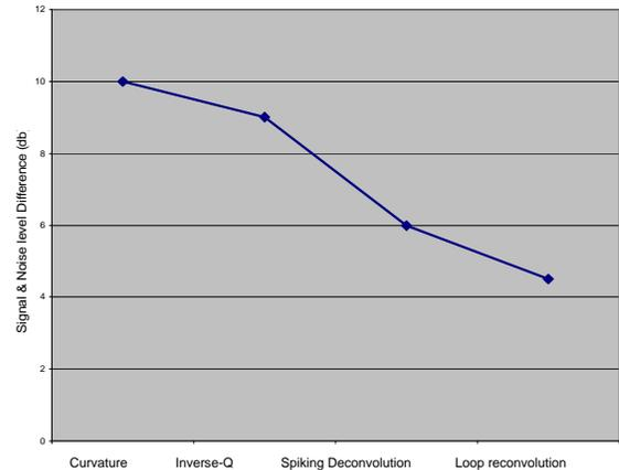
Figure 11: Comparison of noise level between different methods
