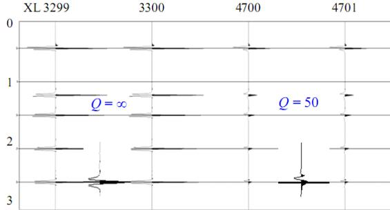
Fig 3 The conventional migration result, it recovers the geometrical spreading, but not the absorption effect.
