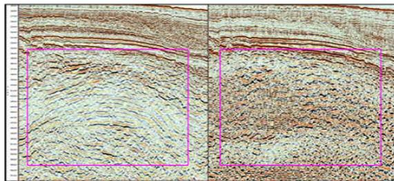
Figure-3(a) & Figure-3(b) are the final PreSTM stack Sections after reprocessing & with vintage processing of a 2D part profile
