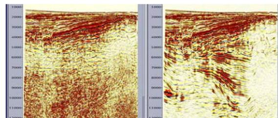
Figure-5(a) & Figure-5(b) are the Final PreSTM & PreSDM (Beam Migration) sections of a 3D line flipped.
