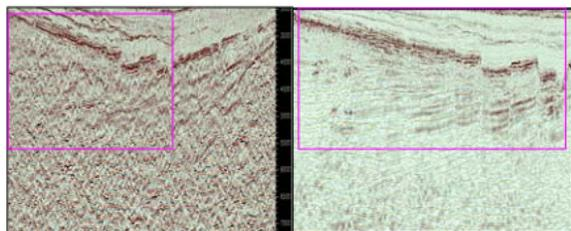
Figure-4(a) & Figure-4(b) are the final PreSTM stack Sections of 2D reprocessed data & a 3D line overlying the same 2D part profile.
