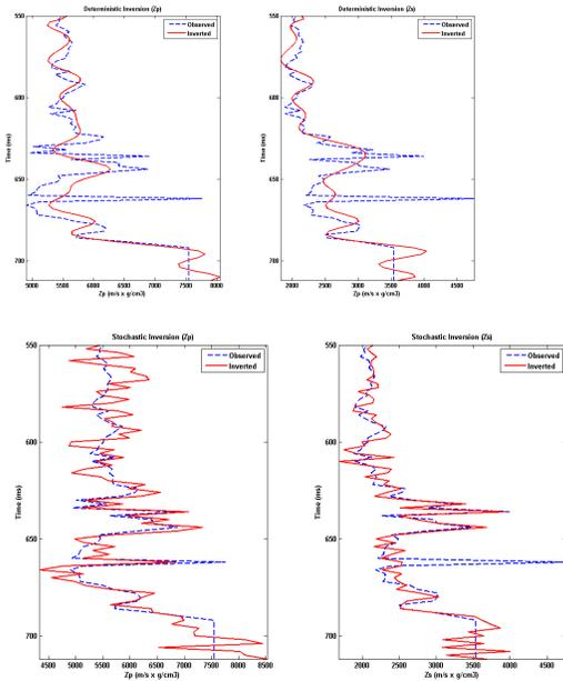
Figure 4: Pre-stack inversion results: AI and SI estimates from a deterministic (top) and fractal based stochastic (bottom) inversion (from Srivastava and Sen 2009).
