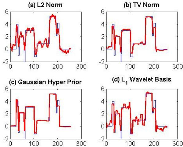
Figure 3: Inversion of seismic data for AI using different regularization techniques. The true model is shown in black while the inverted models are shown in red. Note the superior performance of Gaussian hyper-prior compared to other well known regularization method (from Routh et al 2008).
