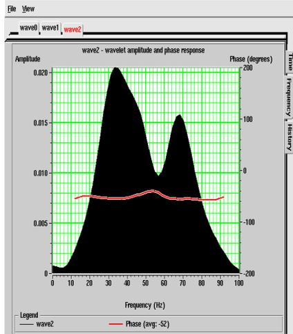
Figure 1: A typical wavelet (top panel) derived from a seismic trace and its corresponding amplitude spectrum (bottom panel). Note the missing low- and high-frequency bands in the spectrum.
