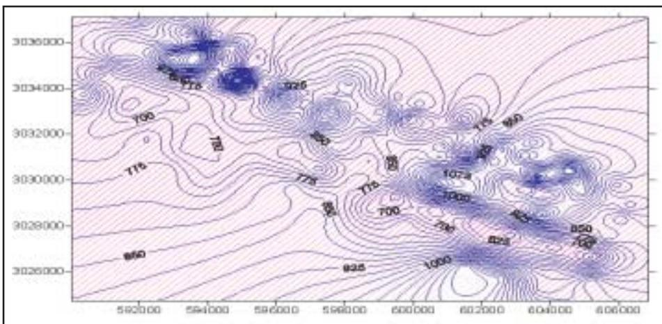
Fig. 8: Velocity model for 2<sup>nd</sup> layer
