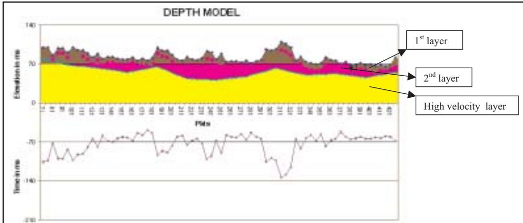
Fig.11 : Depth model Layer-1, Layer-2, Layer-3.
