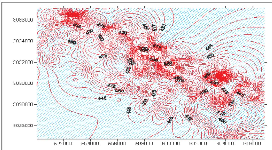
Fig. 7: Velocity model for weathered layer (1<sup>st</sup> layer)
