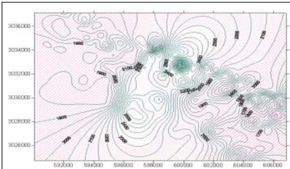
Fig. 9: Velocity model for 2<sup>nd</sup> layer.
