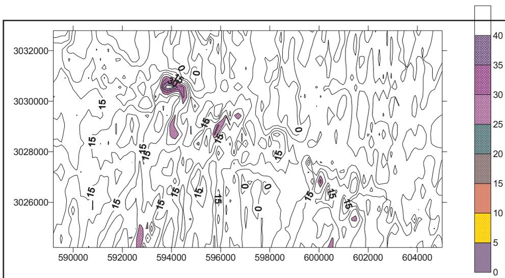
**Fig. 5:** Contours of weathered layer thickness
