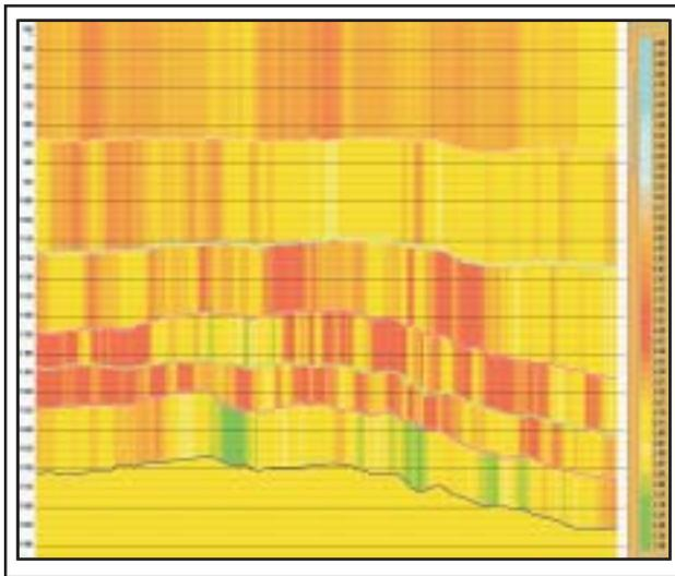
**Fig. 2 :** Time section showing interval  $V_p/V_s$  values calculated using PP and PS isochrons.
