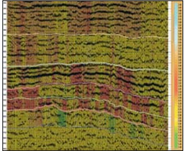
**Fig. 3 :** Time section showing interval  $V_p/V_s$  values with wiggle PS seismic data superimposed.
