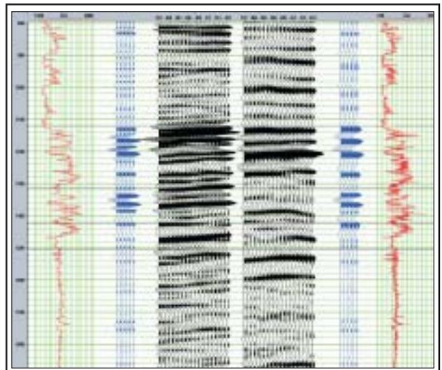
Fig. 1: Correlation of vertical (left) and radial (right) components through PP and PS log-based synthetic modeling, (for better visibility only P- and S-wave logs are shown).
