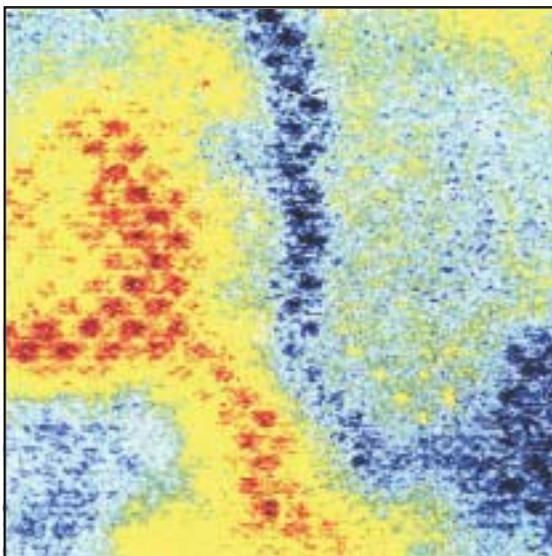
Fig.1a: Acquisition footprints in Land data:- Source lines of Double Zig-Zag geometry are visible.
