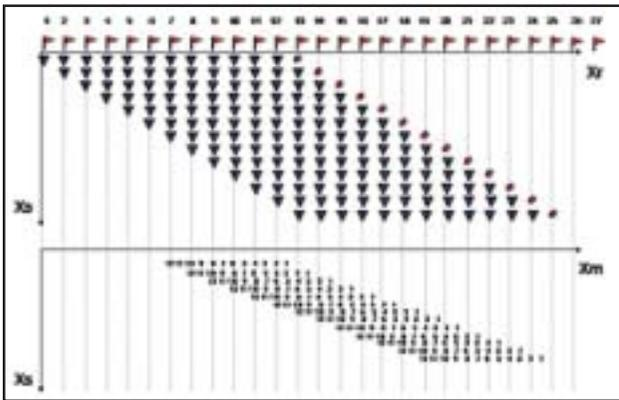
Fig.2a: Stacking diagram for 12 Channels End-on geometry with shot at each picket. Note the offset sampling of odd and even CMP
