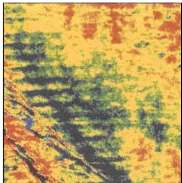
Fig.1b : Amplitude footprints in 4/4 geometry of streamer survey.
