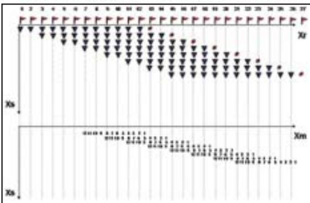
Fig.2b: Stacking diagram for 12 Channels End-on geometry with shot at each alternate picket. Note the four type of offset sampling of CMP.
