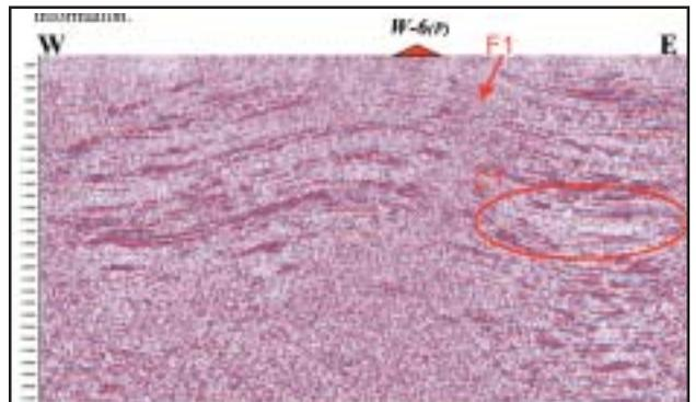
Fig.12. Pre-stack Time Migrated Section of Line B-B'
