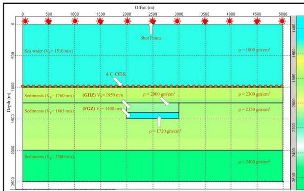
**Fig.1:** Key Model used for anisotropic simulations, Gas Hydrate Zone (GHZ) & Free Gas Zone (FGZ) are located at 1250-m and 1400-m depth respectively. 4C Ocean Bottom Seismometers are deployed on the ocean surface. 20 kHz shot are located at 10-meter depth.
