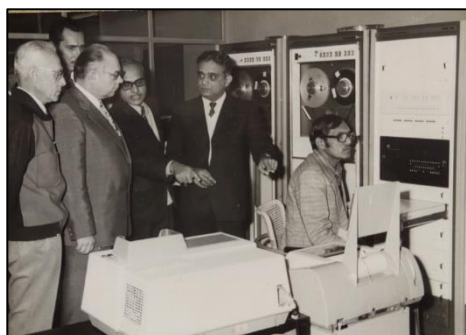
Mr. V. C. Mohan briefing a visiting delegation to the ONGC computer center about the TIOPS components (1972). To the left are the two tape drives, and to the right are the CPU in black, with the FFT box above and the hard disk below. In the foreground is the card reader (left) and teletype printer (right). (Photo courtesy: Mr. V. C. Mohan)
