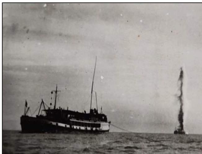
The shooting of a seismic survey in action (1963), with M. V. Mahindra in the foreground and the streamer trailing it. To the right is a waterspout generated by the explosive in water with the shooting boat to the side. (Photo courtesy: Mr. V. C. Mohan)
