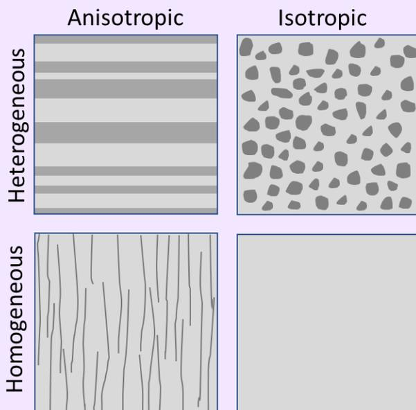
Figure 1: Illustration of the distinction between isotropic, anisotropic, homogeneous, and heterogeneous rock samples.
