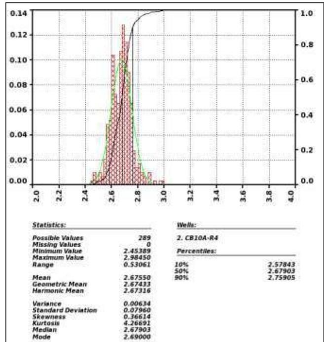
Fig. 4: Histogram of Grain density from NMR log in well B
