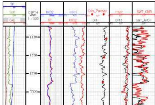
Fig. 5: Log motif of study area showing porosity and water saturation in well B
