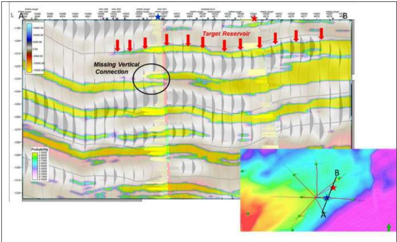
**Fig. 4:** An arbitrary line passing through water injector well (blue star) and the benefiter well (red star) shows seismic and reservoir probability distribution (yellow) in the background at target reservoir level. Geostatistical inversion driven geobody is highlighted in yellow. The continuity at reservoir level is marked by red arrows.
