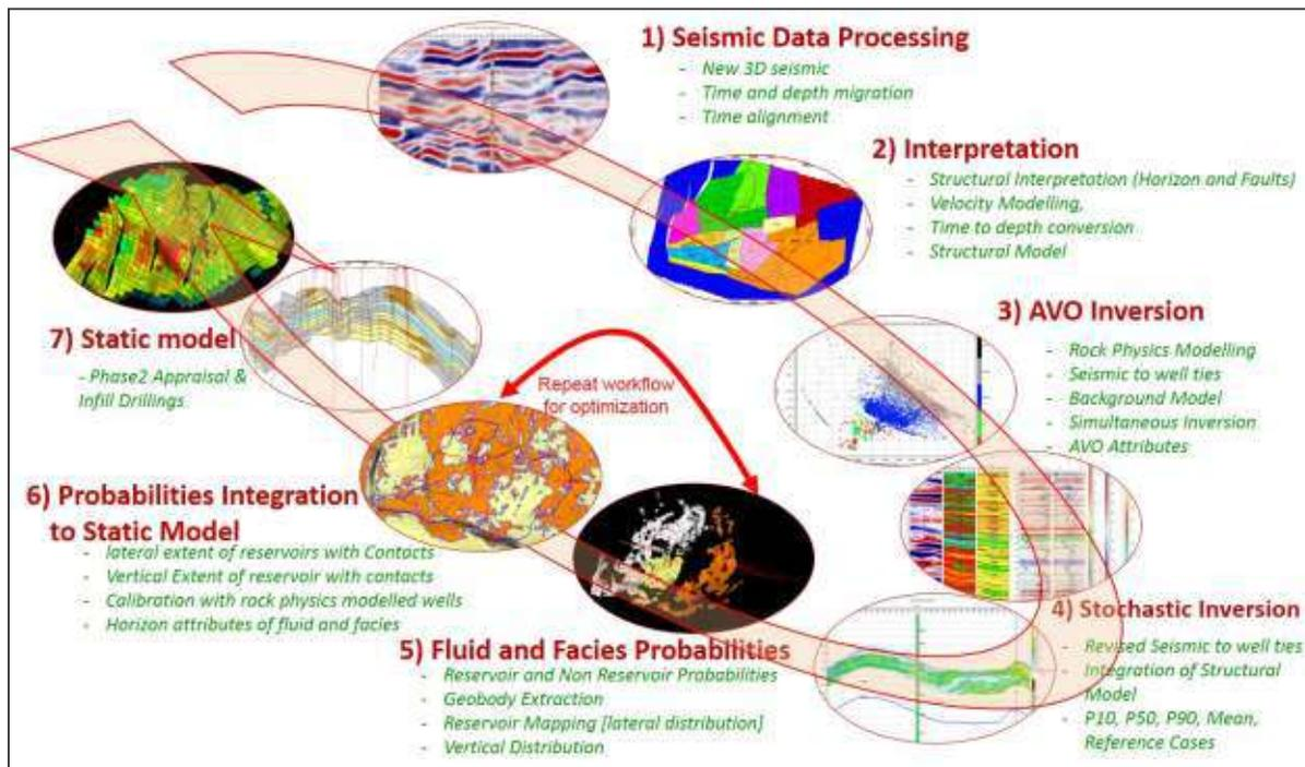
Fig. 2: Stochastic inversion to Static Model integration workflow
