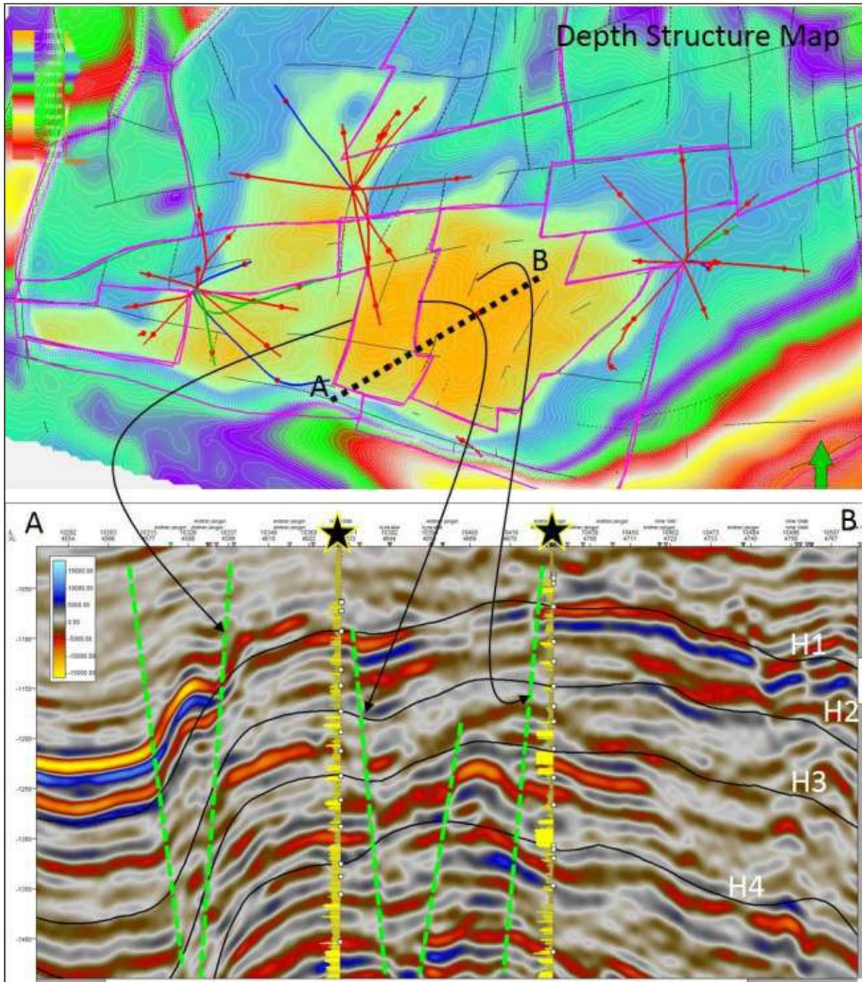
**Fig. 1:** Fault blocks and corresponding seismic line highlighting the complex structural regime. Different fault blocks are demarcated by major faults in the study area and represented by pink color polygons (upper part), minor faults inside the blocks are marked by thin black lines; Seismic section shows major horizons, faults, and two wells showing gamma ray logs (lower part).
