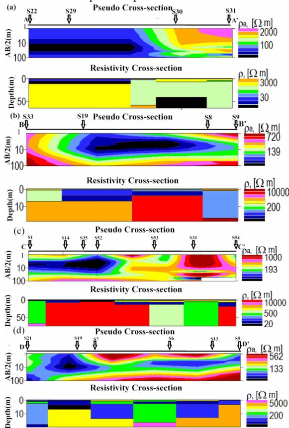
Figure 5: 2D-Resistivity structure along profile (a)AA' (contains sounding point S22-S31); (b)profile BB' (contains sounding point S33-S9) (c) profile CC' (contains sounding point S1-S54);(d) profile DD' (contains sounding point S21-S5)
