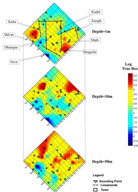
Figure 3: True resistivity contour map at different depth of the study area.
