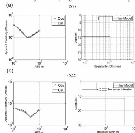
Figure 4: One dimensional inversion of Schlumberger vertical electrical sounding (VES) of station S7 and S22 of the study area. S22 shows the sea water intrusion site.
