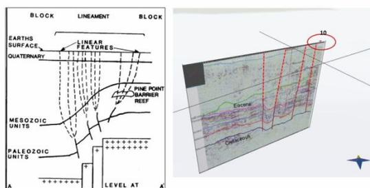
Fig 4: A. Shurr, 1982 Model showing basement faults continuous up to surface in a sub seismic resolution branching out midway and B. in a similar way faults mapped in seismic in Easter Offshore maximum upto Eocene assumed continuous up to surface sub seismically where it coincides with area of seepage repetition.
