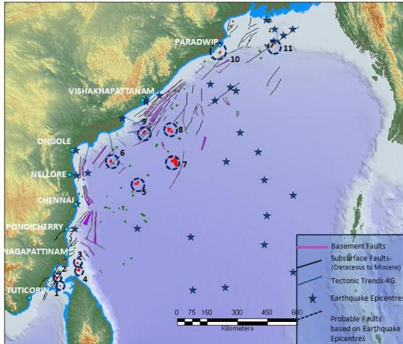
Fig 3: Hydrocarbon seepages and their repetitions correlated with faults mapped using seismic data and earthquake epicenters in the Eastern Offshore. Here areas of seepages are marked in green whereas the areas of seepage repetitions are marked in red
