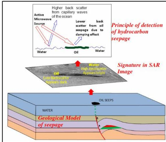
Fig 1: Principle of occurrence of hydrocarbon seepage on an ocean surface and its detection in SAR images: Hydrocarbon leaking out of reservoir to the sea floor along a fault and subsequently floating up to sea surface. At sea surface, backscattering from oil much less than surrounding sea water resulting in oil appearing dark in a SAR Image compared to water
