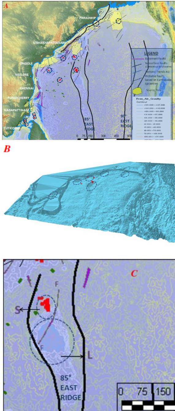
Fig 5: A. seepages correlated with faults and source pods showing most seepage repetitions associated with faults that are attached to source pods B. 3D perspective model of Free Air Gravity of eastern offshore showing seepage repetitions associated with areas of gravity lows that might have acted as kitchens. C. Seepage repetition associated with a gravity low and fault in 85 E Ridge suggesting the existence of a petroleum system
