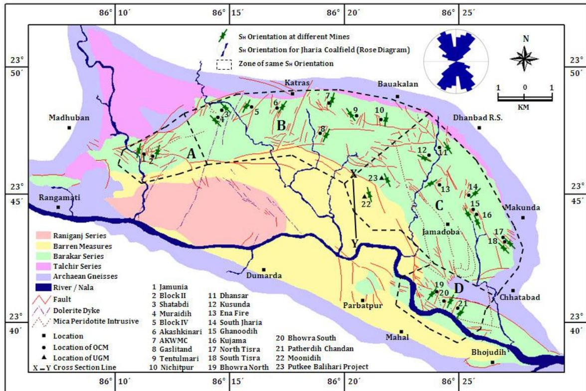
**Figure 1:** Stratigraphic and structural map of Jharia coalfield (after Sengupta, 1980) showing locations of opencast and underground coal mines and in-situ stress orientation of Jharia coalfield, India. Mean  $S_H$  orientation displayed in rose diagram is mostly N-S varying NNE to NNW.
