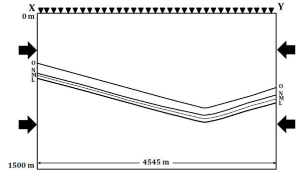
**Figure 3:** 2-D model for the X-Y section. Four coal seams (L, M, N and O) are identified. Model is constrained at the top boundary, and solid arrows indicate the applied stress.
