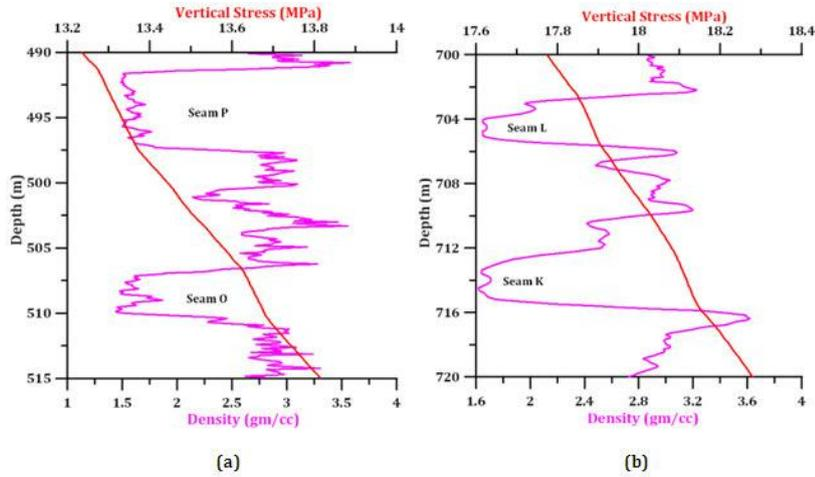
**Figure 2:** Density log signature from a CBM well indicates the major coal seams and the variation of vertical stress with depth against the identified coal seams.
