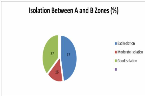
The above pie chart extends the concept of gas migration from Mukta to Bassein through channelling behind casing phenomenon and since 20 wells (47%) have poor isolation i.e. BA-1,2,5,6; BB-4,5,7,8,9; BD-2,3,4,5,6 and BE-2,5,8,9. Mukta production is understandably in vogue from almost all platforms.
