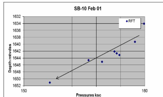
Figure-3: Pressure vs. Depth of Mukta
