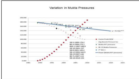
Figure-4: Variation in Mukta Pressures with Time
