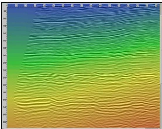
Figure-10: Composite display of RMS velocity and stack Section (TWT: 800-4000ms)
