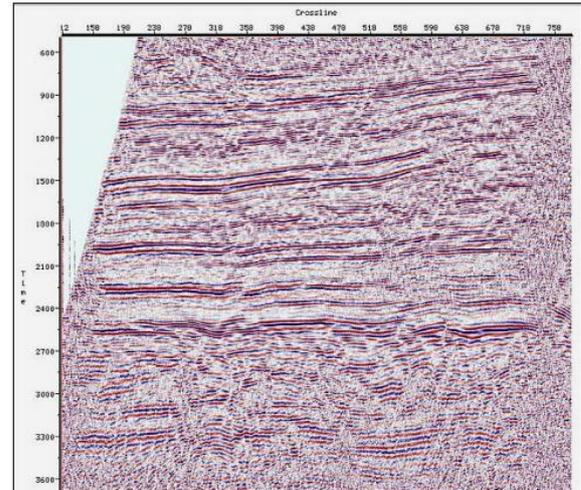
Figure-3: Auto-static applied NMO Stack
