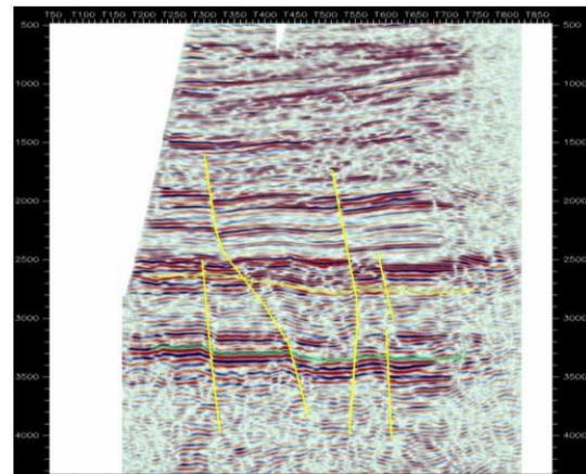
Figure-12: Horizon / fault interpreted PSTM section of IL-164
