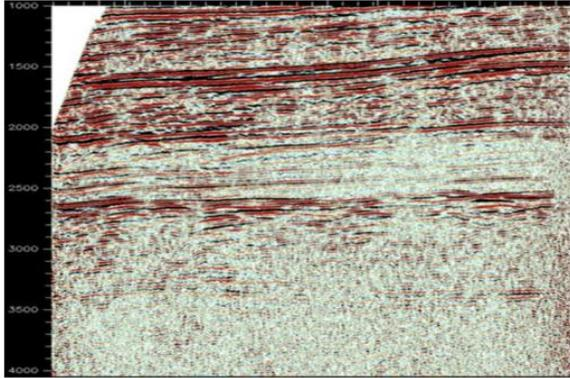
Figure-8: Conventionally (NMO+DMO+ Post stack migration) Processed Section
