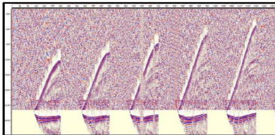
Figure-2: Geometry merging QC (LMO)
