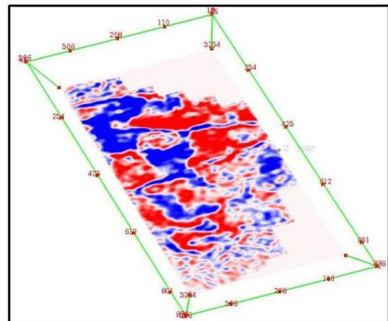
Figure-13: Time Slice at Tura formation (Time: 3300 ms.)
