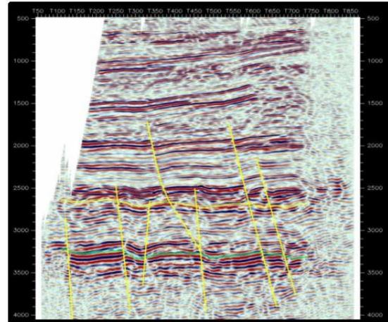
Figure-11: Horizon / fault interpreted PSTM section of IL-250
