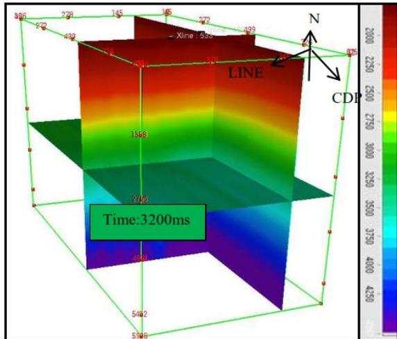
Figure-5: Cross Sectional View (IL: 250 & XL: 500) from the RMS velocity volume
