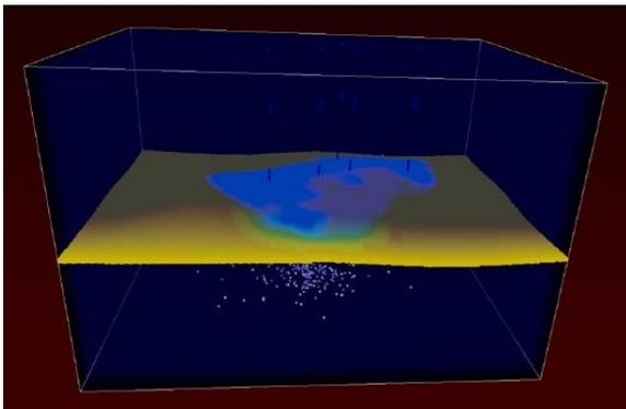
Figure 5: Velocity at the reservoir using reflection tomography for the reservoir top, well data for its thickness, and passive seismic for tuning the velocity estimate.
