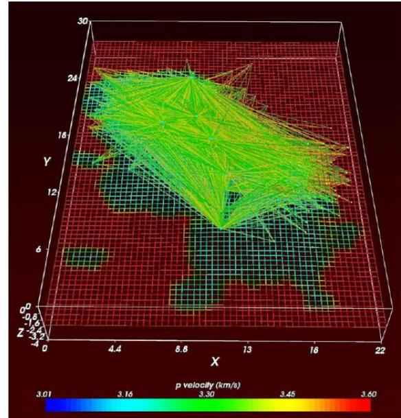
Figure 2: The available ray paths for seismic tomography cover only part of the gas reservoir.
