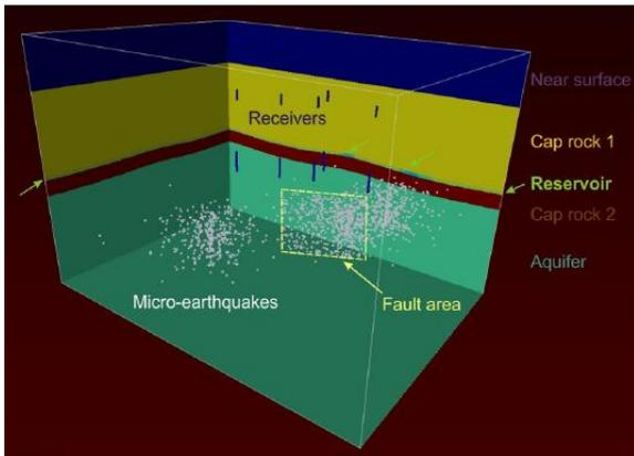
Figure 1: 3D view of the synthetic model that mimics the In-Salah test site.
