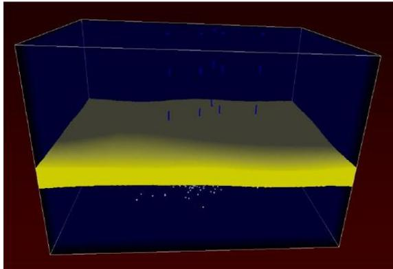
Figure 4: Estimated velocity in the reservoir vicinity by 3D Reflection tomography.
