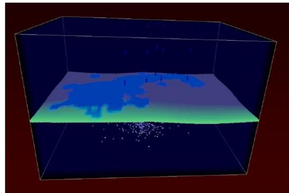
Figure 3: 3D view of the layer with the gas reservoir only. The white dots show some of the micro-earthquake hypocenters.
