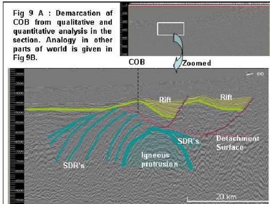
Fig 9 A : Demarcation of COB from qualitative and quantitative analysis in the section. Analogy in other parts of world is given in Fig 9B.
