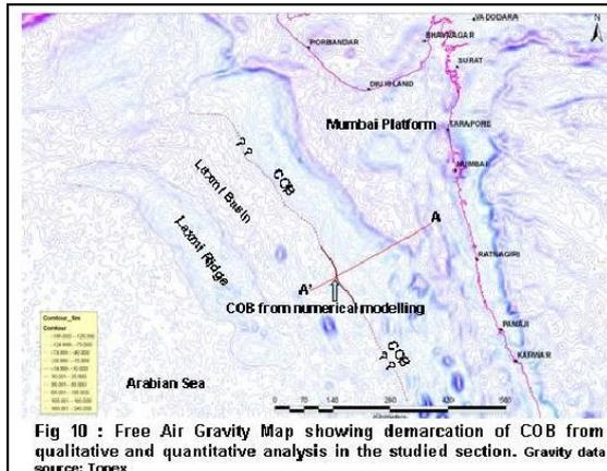
Fig 10 : Free Air Gravity Map showing demarcation of COB from qualitative and quantitative analysis in the studied section. gravity data source: TOPEX
