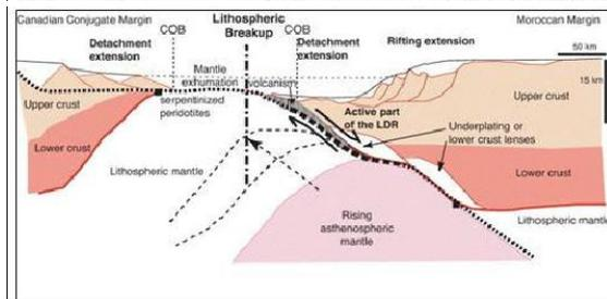
Fig 9B :2D-Model of the conjugate margins of Morocco and Nova Scotia demarcating COB. Ref: Maillard Agnes et. Al, 2006
