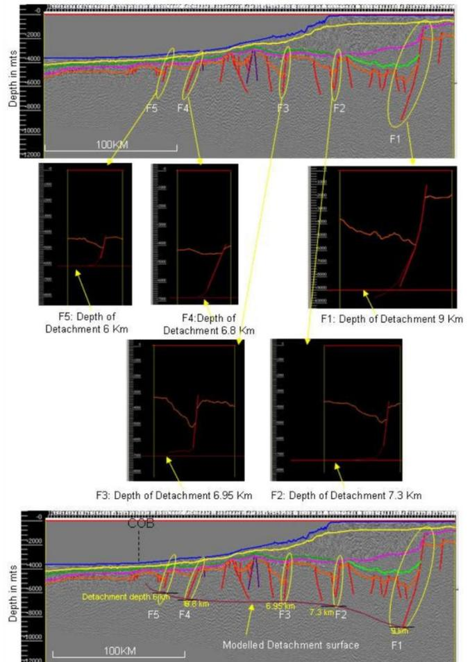
Fig 8: Determination of detachment depth using Move software by MVE and finally determining the modeled detachment surface.
