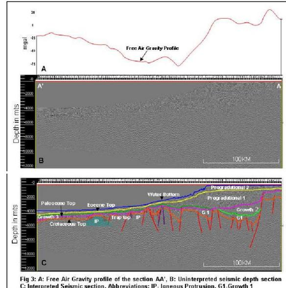
Fig 3: A: Free Air Gravity profile of the section AA'; B: Uninterpreted seismic depth section C: Interpreted Seismic section. Abbreviations: IP: Igneous Protrusion, G1:Growth 1
