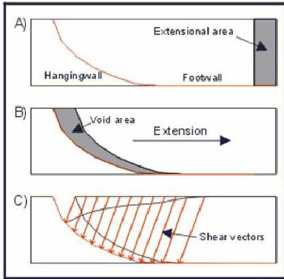
Fig 7: Principle of Inclined shear. A) Initial state showing amount to be extended B) Area of extension equals to area of void C) Shear vector controls how hanging wall elements collapse down onto fault plane. Ref: MOVE by M/S MVE
