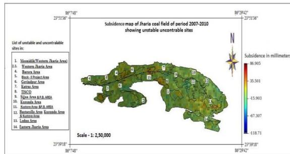
Figure 6 b: Subsidence maps of the Jharia coalfield showing the unstable, uncontrollable sites in Jharia coalfield for the image pair 2007-04-21/2010-01-30.
