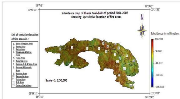
Figure 5 a: Subsidence map of the Jharia coalfield showing the speculative location of fire areas in different collieries for the image pairs 2004-05-01 /2007-04-21
