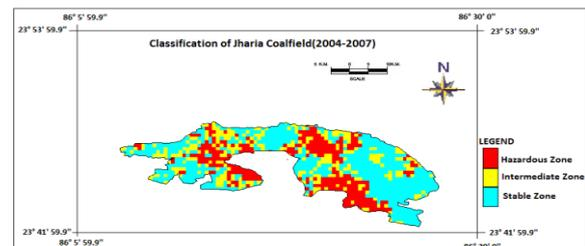
Figure 4 a: Classification image of Jharia coalfield for 200405-200704 interferometric pair showing hazardous zone in the coalfield.
