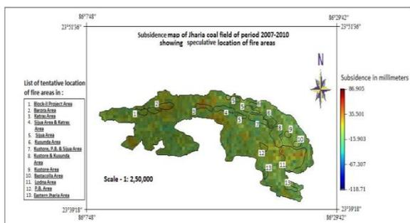
Figure 5 b: Subsidence map of the Jharia coalfield showing the speculative location of fire areas in different collieries for the image pairs 2007-04-21/2010-01-30
