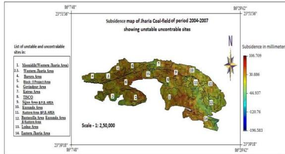
Figure 6 a: Subsidence maps of the Jharia coalfield showing the unstable, uncontrollable sites in Jharia coalfield for the image pair 2004-05-01 /2007-04-21
