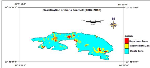
Figure 4 b: Classification image of Jharia coalfield for 200704-201001 interferometric pair showing hazardous zone in the coalfield.
