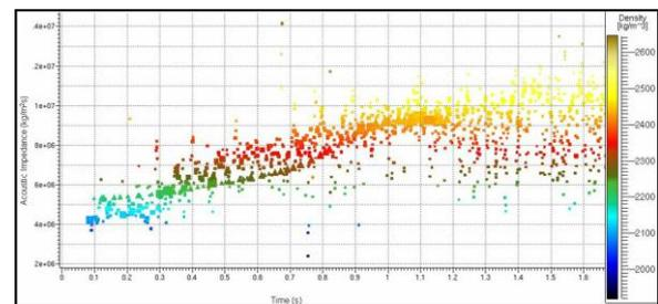
Figure 3: Cross-plot of Acoustic Impedance (AI) from well X and from interval velocities (estimated by processing workflow) colour coded by density.
