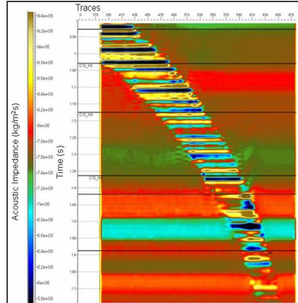
Fig. 5 Absolute impedance model calculated by seismic inversion. Dark blue colour is used for soft sediments (lower absolute acoustic impedance) and yellow represents the hard sediments (increasing acoustic impedances).
