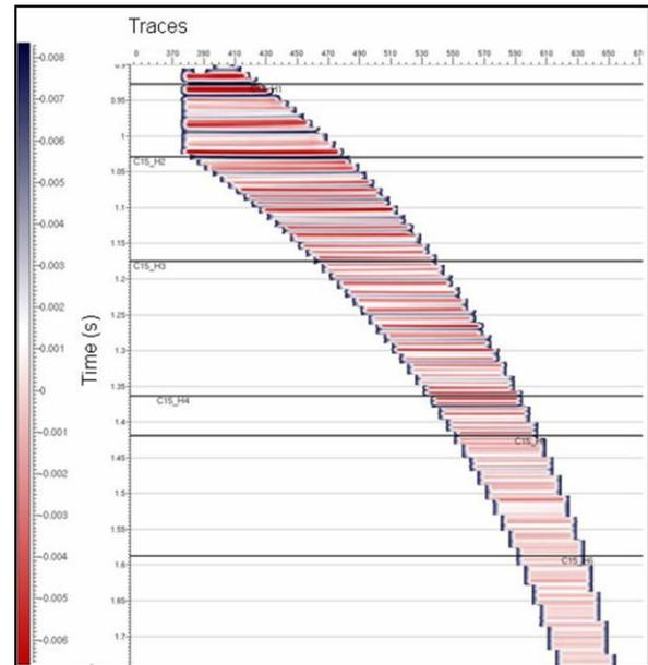
Figure 2: Example of an interpreted VSP section
