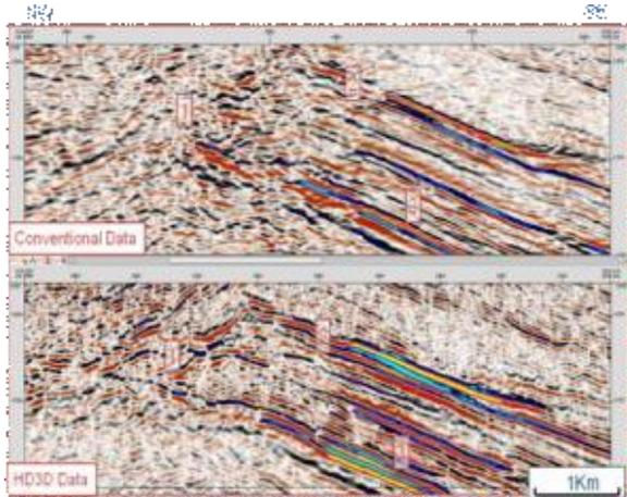
Figure 2: HD (high density) 3D data was acquired in 2006-07 with 10m x 10m station interval (Mangala field). High trace density data has demonstrated the better imaging of faults, events and also higher resolution within reservoir interval.
