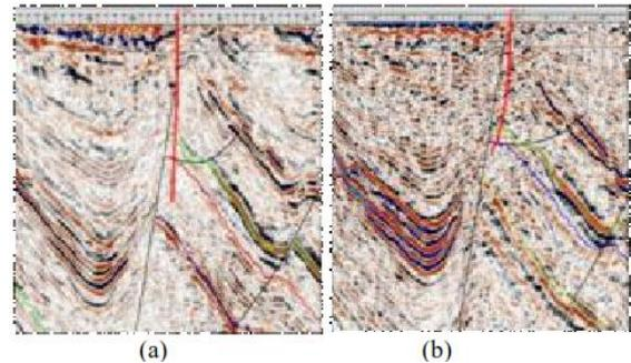
Figure-4: Objective oriented PSTM reprocessing has helped in better imaging of the crestal part in the Bhagyam field. This has resulted in change of the initial positioning of B1-PS8G location to up-dip side.
