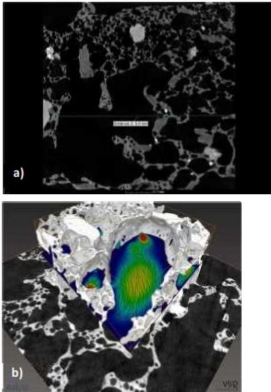
Figure 4: (a) 2-D image through the reconstructed volume of a pyroclastic rock (view width: 5 mm). The right hand image (b) visualizes in 3D the results of fluid flow modelling performed by Avizo software.
