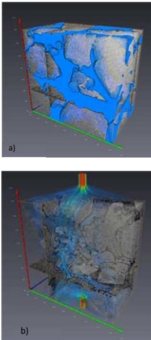
Figure 2: 3-D visualization of segmented microporosity within the scanned Bentheimer Sandstone (a) and streamline visualization of fluid flow (b) within this void space derived by Avizo (VSG).
