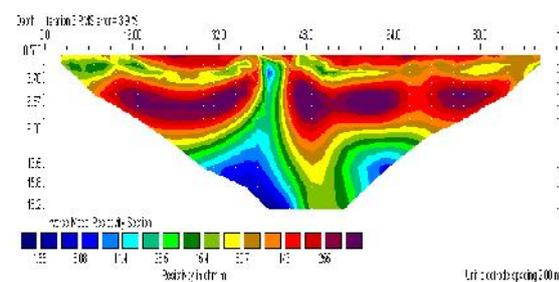
Fig. 2a True resistivity section along Profile AB (Fig.1)
