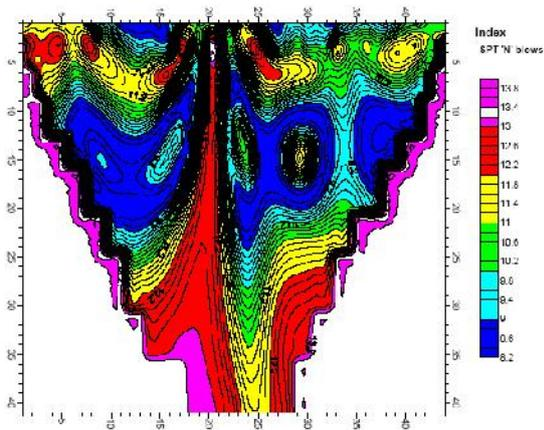
Fig. 4b Predicted 2-D SPT section as per our methodology
