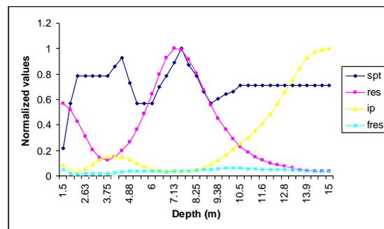
Fig. 3b Normalized plots of true resistivity, IP chargeability, fictitious resistivity and SPT 'N'
