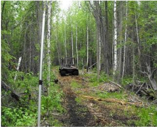
Figure 2: Use of hyMesh option on Sigma system to obtaining passive data in low channel density thick forest conditions, allowing high band width real time data transfer of “uncommitted data ” without cables.
