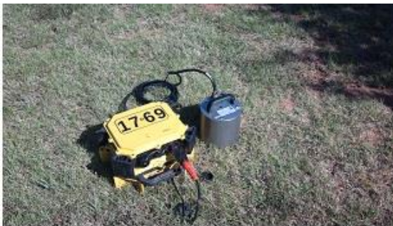
Figure 3: Use of high sensitivity sensor (Guraltype) with standard Sigma cable less system. A very important feature of modern instrumentation for passive is that they can handle a wide variety of sensors.
