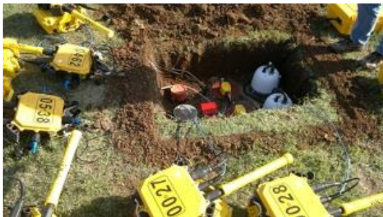
Figure 13: Testing of different passive and powered sensors, data transferred by WiFi in this case. Courtesy Spectrase and iSeis Cos.
