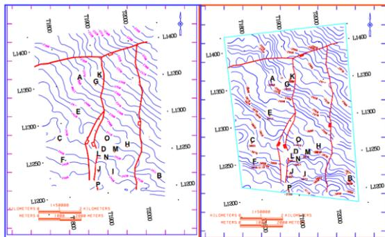
Figure 9(a): Time Map at GS-1 Top (b) Structure Map at GS-1 Top
