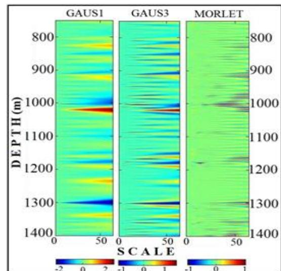
Fig.11. Scalograms of the Neutron log of Well-B generated using Gaus1, Gaus3 and Morlet wavelets.
