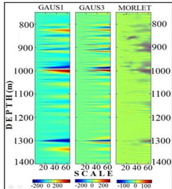
Fig.10. Scalograms of the Gamma-ray log of Well-B generated using Gaus1, Gaus3 and Morlet wavelets.
