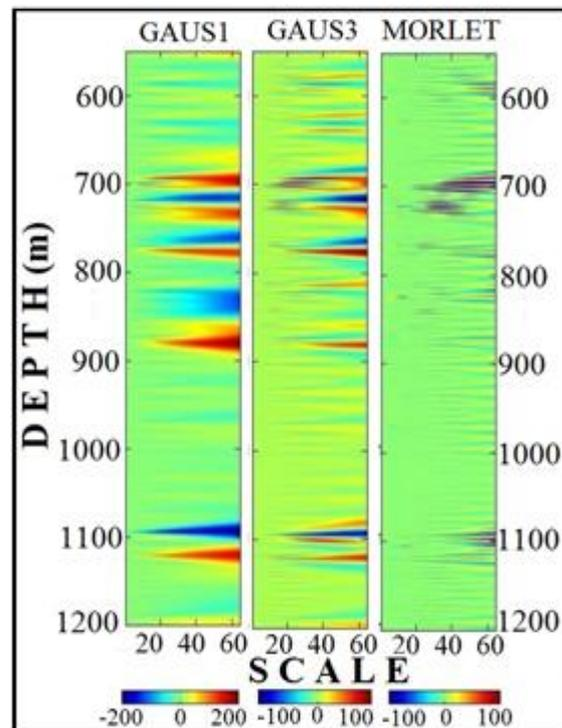
Fig.7. Scalograms of the Gamma-ray log of Well-A generated using Gaus1, Gaus3 and Morlet wavelets
