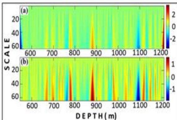
Fig.5.Example of scalogram plots of CWT analysis of neutron porosity log data of Well-A, when edge effects in the signal are not removed (a) and removed (b).
