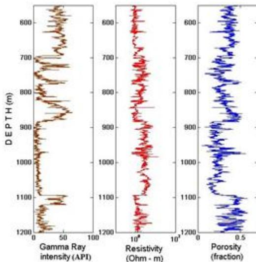
Fig.2. Gamma-ray, Resistivity and Neutron porosity logs of Well-A.
