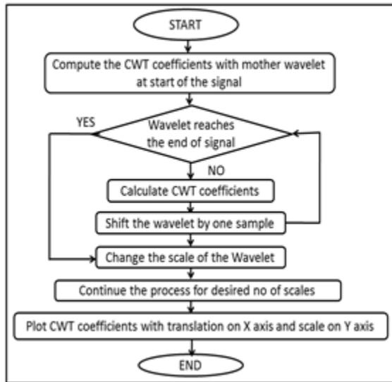
Fig.4.Flow chart for Continuous wavelet transformation.
