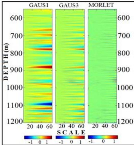
Fig.8. Scalograms of the Neutron log of Well-A generated using Gaus1, Gaus3 and Morlet wavelets.
