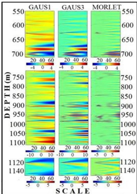
Fig.9. Scalograms of the Resistivity log of Well-A generated using Gaus1, Gaus3 and Morlet wavelets.
