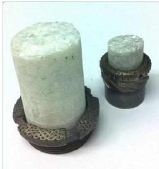
Figure 1: Comparison of the large-format SWC (1.5”x3”) with conventional rotary SWC (~1”x2”)
