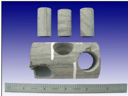
Figure 2: Large-format SWC subsampled on three axes for geomechanical testing (Ref: Laronga, 2011).
