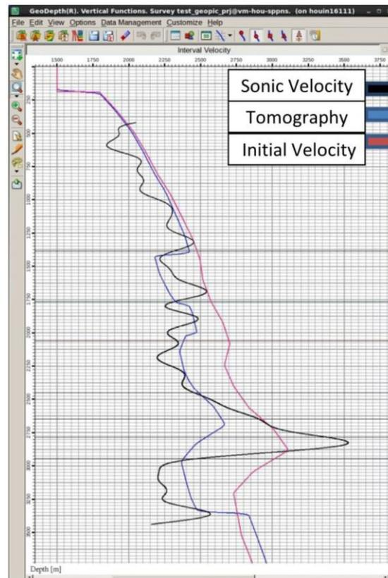
Fig.7: showing comparison of velocity before and after welltie Tomography with Sonic velocity. Note the good match between Sonic and welltie velocity.
