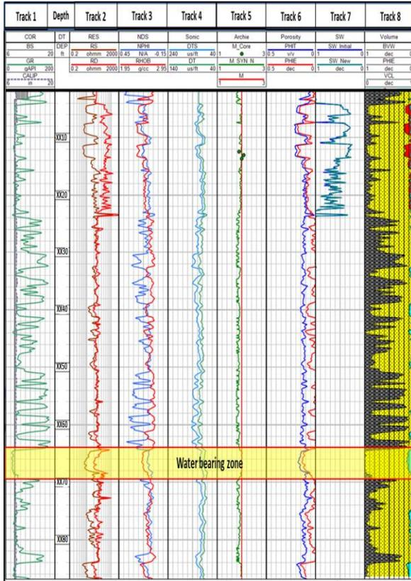
Figure 5: Log plot showing comparison of water saturation estimated using constant cementation exponent (Track 7 blue curve) and cementation exponent estimated from aspect ratio (Track 7 green curve)
