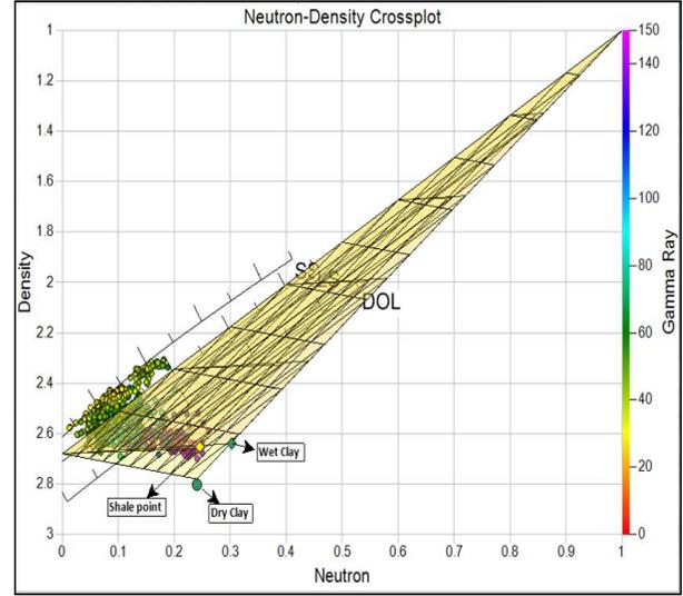
Figure 2: Density-Neutron crossplot showing wet and dry clay points.
