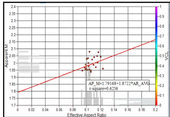
Figure 4: Cross-plot of effective aspect ratio and cementation exponent (apparent m) computed in water bearing zone
