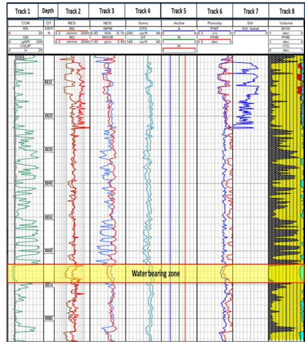
Figure 3: Log plot showing water saturation (Track 7 blue curve) estimated using constant cementation exponent (Track 5 red curve)
