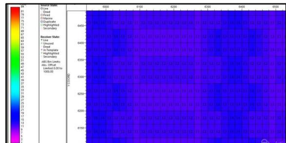
Fig.11: Number of traces is 11-14 for offset range of 0-1000 m in option-3
