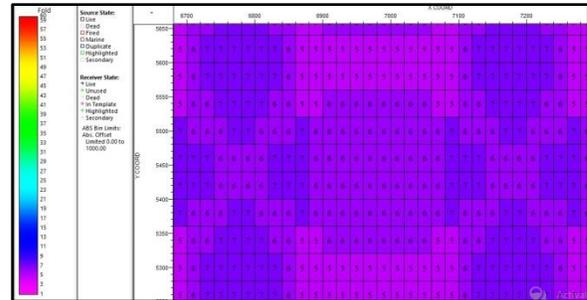
Fig.9: Number of traces is 5-7 for offset range of 0-1000 m in option-1
