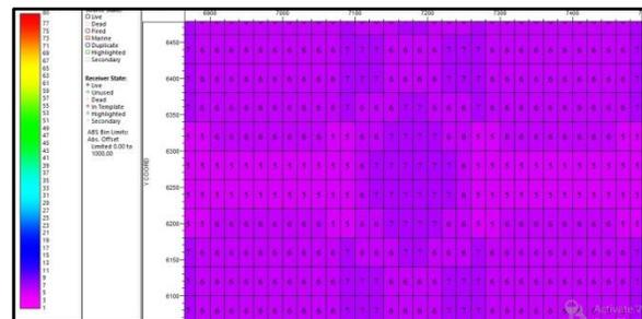
Fig.10: Number of traces is 5-7 for offset range of 0-1000 m in option-2
