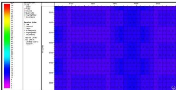
Fig.14: Number of traces is 11-14 for offset range of 0-1000 m in option-4
