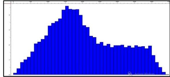
Fig.14: Histogram for option-3 shows considerable traces are available beyond offset of 4000m.
