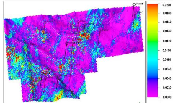
Fig.6 Computed Fracture porosity for Nohta-B gas bearing layer
