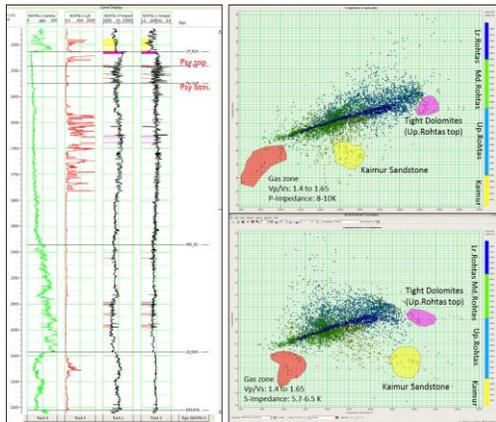
Fig.4 Impedance (P&S) and Vp/Vs response of Nohta-A gas zone in Upper Rohtas
