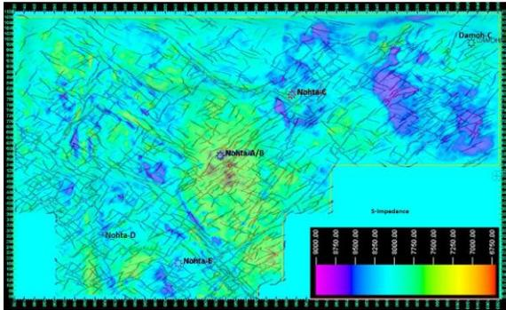
Fig.7 Prospective fracture corridors for Nohta-B gas bearing layer (Upper Rohtas) through ant track and S-impedance maps.
