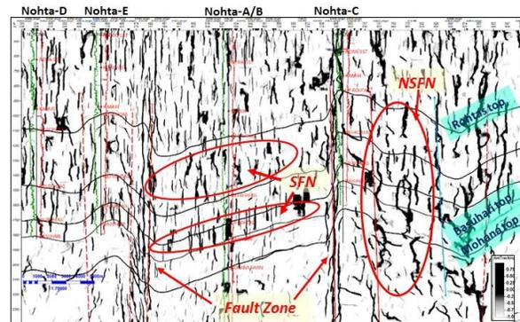
Fig.5 Vertical Ant track section depicting SFN, NSFN and fault induced fracture network within Rohtas Formation in Nohta-Damah area.
