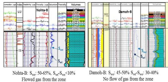
Fig.9: Paralogs of tested zones in Nohta-B and Damoh-B showing the effects of bound water on gas flow behaviour.
