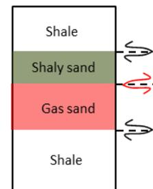
Figure 5: Schematic diagram of a scenario where a peak over trough situation is encountered. The impedance of shaly sand is higher than shales resulting in peak signature at top interface.
