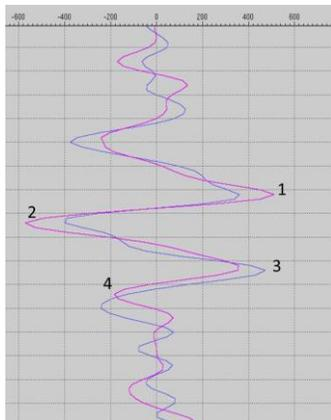
Figure 11: Seismic trace profile from a cdp at a proposed location from case study. Near angle is in blue far angle is in pink color.
