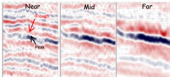
Figure 8: Seismic data from Near, Mid and Far angle stacks. The bright spot is characterised by trough over peak anomaly. The anomaly is not seen at near angle stack but appears at far angle stack.
