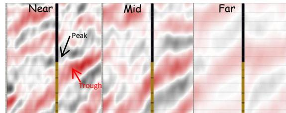
Figure 6: Seismic data from Near, Mid and Far angle stacks overlain by facies log (black represents shale while brown represents gas sand). The bright spot is characterized by peak over trough anomaly in near stack data which changes to trough in far data after polarity reversal of amplitude.
