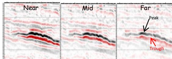
Figure 3: Seismic data from Near, Mid and Far angle stacks. The bright spot is characterised by peak over trough anomaly.
