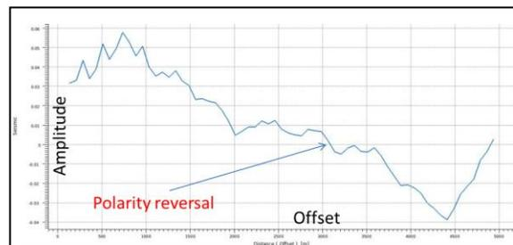
Figure 7: Amplitude Variation with offset curve at the location of peak shown in the section from Figure 6. Presence of polarity reversal can be seen as the amplitude changes from positive to negative values.
