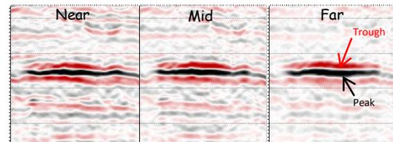
Figure 4: Seismic data from Near, Mid and Far angle stacks. The bright spot is characterised by trough over peak anomaly.
