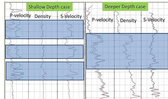
Figure 2: A fluid substitution study showing p-velocity, density and s-velocity logs for 100% water (blue color) and 10% gas (red color) case for shallow depth (left panel) and deeper depth (right panel). The blue boxed portion shows sand zone.
