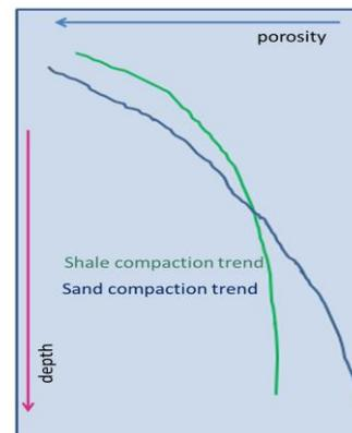
Figure 1: Compaction trends for shale and sand in terms of porosity variation. It can be seen that at certain depth the trends intersect and after that the rate of compaction is more in sands than in shales. The arrows point in the direction of increase in a particular parameter.
