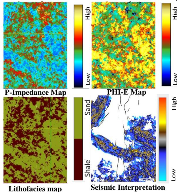
Figure 13. The channel sand as interpreted from seismic amplitude map is also seen in the P-Impedance & lithology map. Also, the result is more pronounced in the Effective Porosity map.
