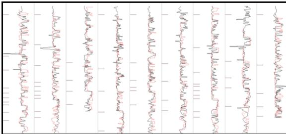
Figure 11: Blind well QC of PHIE. The black curve is that of the well data while the red trace is the simulated PHIE along the well trajectory.
