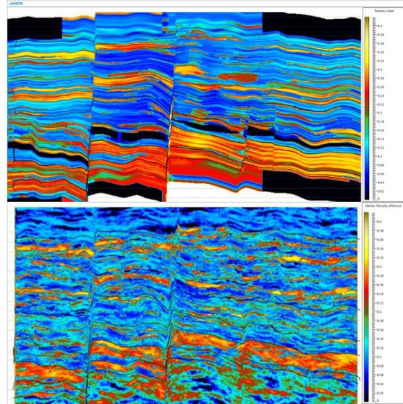
Figure 12: Comparison between the previous static model (top) and one of the geostatistically simulated PHIE volume (below).
