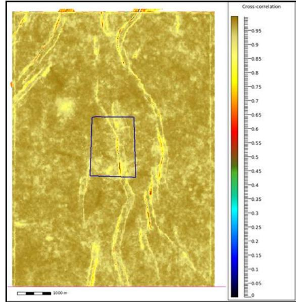
Figure 8: Synthetic-Seismic correlation. The lower values are at the fault locations.
