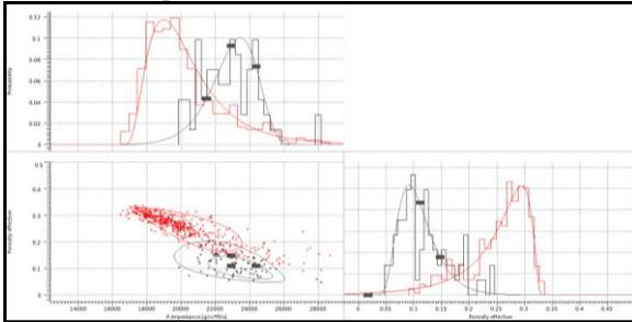
Figure 7: Co-simulation of PHIE and P-Impedance for sand (red) and shale (black) facies.
