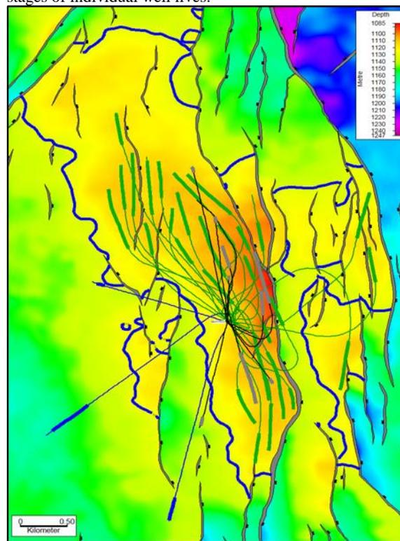
Figure 1: Bualuang Field structure map on top T4.1 (main Reservoir).
