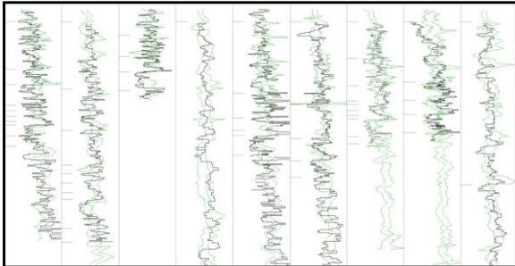
Figure 10: Blind well QC of P-Impedance. The corridor of the green curves displays the mean +/- 1 standard deviation of the P-Impedance along the well trajectory while the black trace is the well log.
