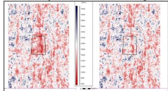
Figure 4: RMS amplitude map of the reservoir zone. Map showing dim amplitude before scaling (left), which was subsequently corrected after scaling (right).
