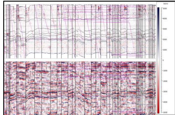
Figure 9: Inverted Residual (above) and input seismic (below). The inversion window between the horizons does not show any residuals.
