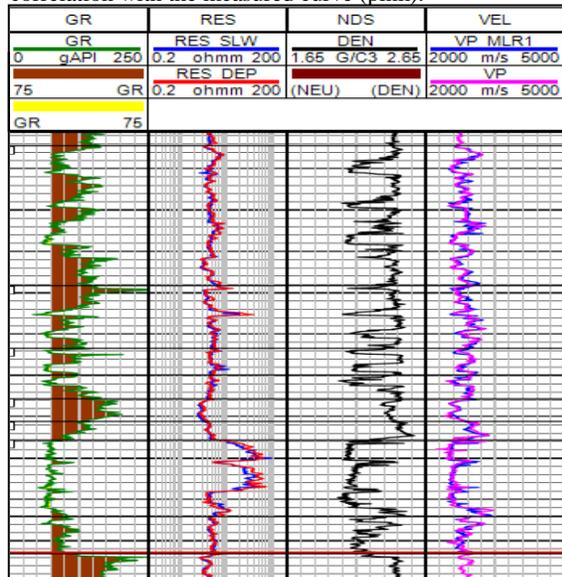
Figure 5: P-wave synthesis via multi-linear regression. The well sonic is displayed in blue in track 4 while the synthesized p-sonic is displayed in pink.
