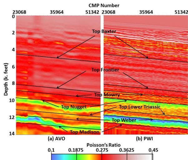
Figure 1: Comparison of the estimated Poisson's ratio from (a) AVO inversion and (b) PWI. Some of the formation tops, interpreted from the RSU-1 well data and RSU geology are also marked.
