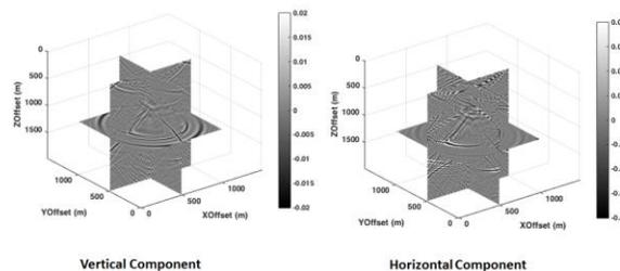
Figure 6: Vertical and horizontal component of response computed using 3D finite element modeling.
