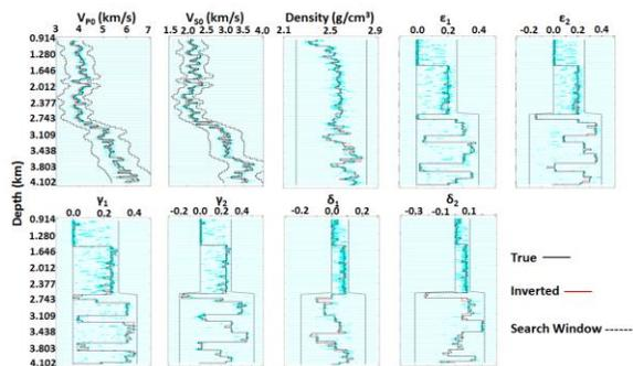
Figure 4: Demonstration of the anisotropic PWI. Estimation of the vertical P- and S-wave velocities ( $V_{P0}$ ,  $V_{PS}$ ), density, and the Thomsen-Tsavankin parameters (Thomsen, 1986; Tsavankin, 1997)  $\epsilon_1$ ,  $\epsilon_2$ ,  $\gamma_1$ ,  $\gamma_2$ ,  $\delta_1$ , and  $\delta_2$  are shown.
