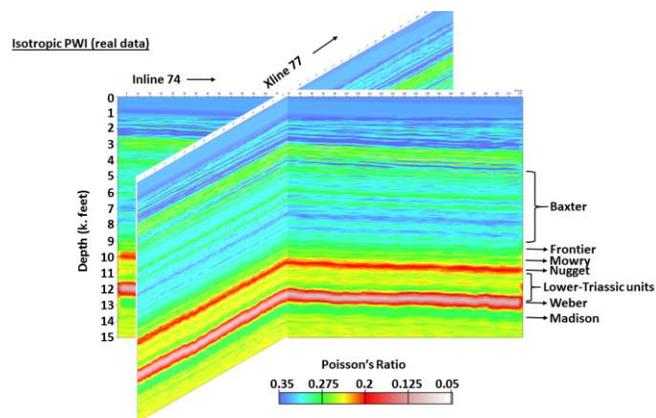
Figure 2: Example of 3D PWI applied to RSU 3D seismic data with interpreted formation tops. Notice the difference in the color scale between Figure 1 and 2.
