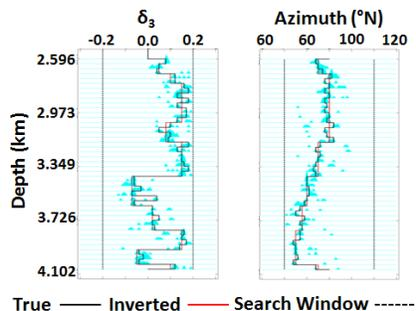
Figure 5: Same as Figure 5 but for the estimation of the Thomsen-Tsavankin parameter  $\delta_3$  and the principal anisotropy direction. Because only the lower part of the model was azimuthally anisotropic, these parameters were estimated and shown only for that part.
