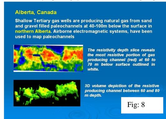
shallow resistivity survey to chase the known gas sand to know its extension. In Alberta such reservoirs were tracked by air borne electromagnetic surveys (fig: 8). As
