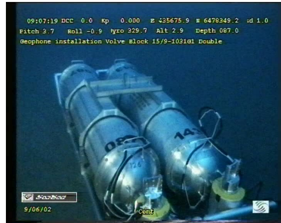
Figure 3: The two nodes coupled to together in order to verify similar coupling responses on records.
